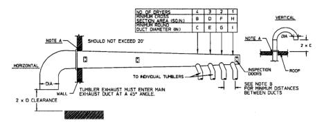
IMPORTANT: NO MORE THAN 4 DRYERS CAN BE CONNECTED TO ONE COMMON DUCT ( VENT ).
