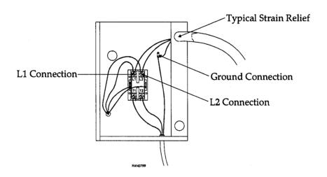
If local codes permit, power to the dryer can be made by the use of a flexible U.L. listed power cord/pigtail (wire size **must conform** to rating of dryer), or the dryer can be hard wired directly to the service breaker panel. In both cases, a strain relief **must be** installed where the wiring enters the dryer.
