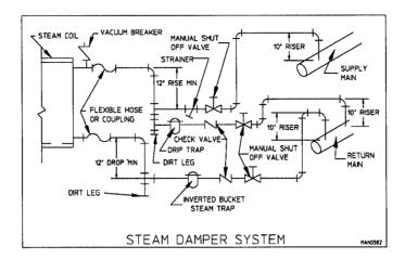
Install an inverted bucket steam trap and check valve at least 12-inches below the steam coil as near to the coil as possible. A vacuum breaker **should be** installed in the piping. This will prevent the condensing steam from causing a vacuum inside the coil possibly damaging the coil. The supply and return lines **should be** insulated. This will save energy and provide for the safety of the operator and maintenance personnel.
