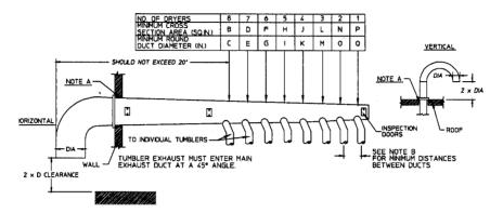
IMPORTANT: NO MORE THAN 8 DRYERS CAN BE CONNECTED TO ONE COMMON DUCT ( YENT ).
