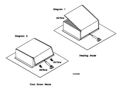
Diagram 2 shows the damper in the cool down (closed) mode, pulling ambient air directly into the basket (tumbler) without passing the coils.
