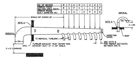
IMPORTANT: NO MORE THAN 8 DRYERS CAN BE CONNECTED TO ONE COMMON DUCT ( VENT ).
